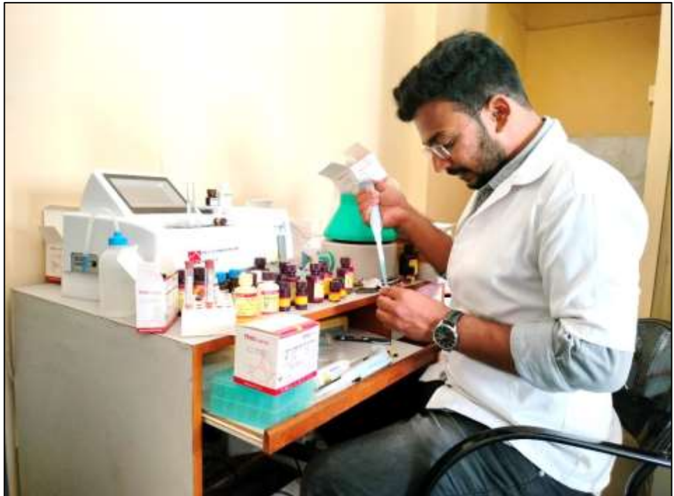
Plate no 3.8 : Analysing serum sample on the Erba Mannheim, CHEM 7, Semi-automated clinical chemistry analyzer.
